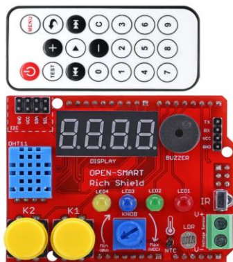
Figure 1: Rich Shield with Infrared (IR) Remote Controller
